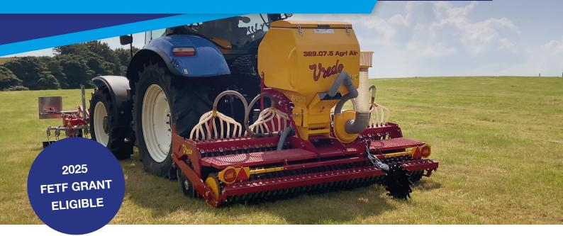
Vredo's direct drill machines are a must for anyone looking for a professional approach to direct drilling in arable stubble such as cereals and cover crops. The unique double-disc system avoids disturbing the soil and is therefore the most environmentally responsible way of drilling. The uncultivated soil remains contain the organic layer and keeps its solidity, humidity, and structure.
